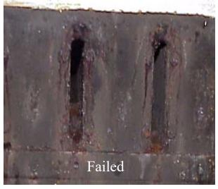
Inspect the inlets of the secondary heat exchanger. If the inlets are significantly obstructed by corrosion or there is significant corrosion and delamination of the polypropylene laminate, replace the secondary heat exchanger.
