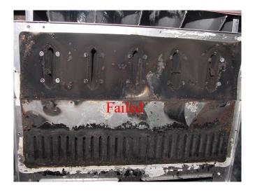
If the coupling box or cold spot baffle has significant corrosion and debris, replace the coupling box. A new cold spot baffle is included in the coupling box kit. Remove the cold spot baffle to reveal the secondary heat exchanger inlets. Clean off any excessive silicone sealant that may be obstructing the passages around the cold spot baffle.
