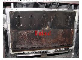
If soot is present on all parts (primary heat exchanger outlet, coupling box and secondary heat exchanger inlet), replace the entire heat exchanger assembly.
