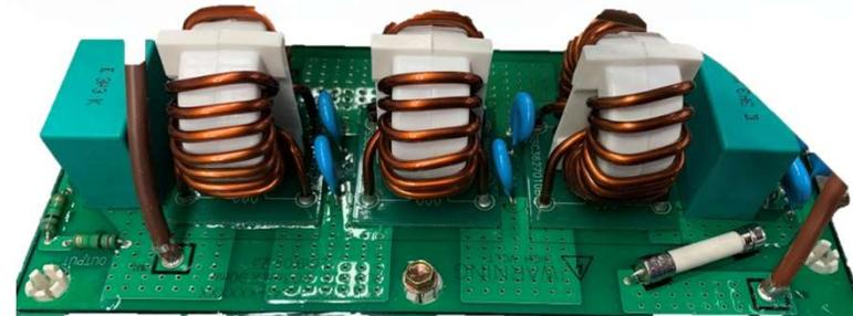
The EMI filter board is intended to block the inherent electrical noise associated with VFD drives from being transmitted over power lines throughout the home.
