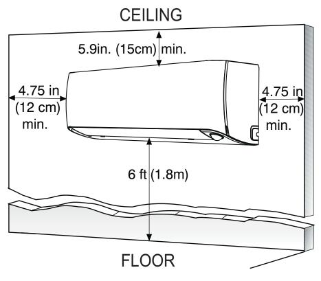
Fig. 3 — Indoor Unit Clearances
