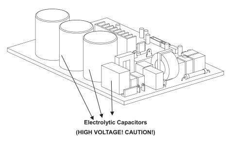
Fig. 13 — Electrolytic Capacitors
