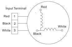
Fig. 22 — Indoor AC Fan Motor
