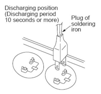
**Fig. 14 — Discharge Position NOTE: Fig. 14 is for reference only. Actual appearances may vary.**
