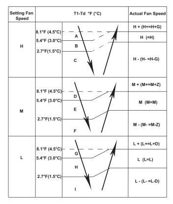
Fig. 27 —Indoor Fan Running Rules
