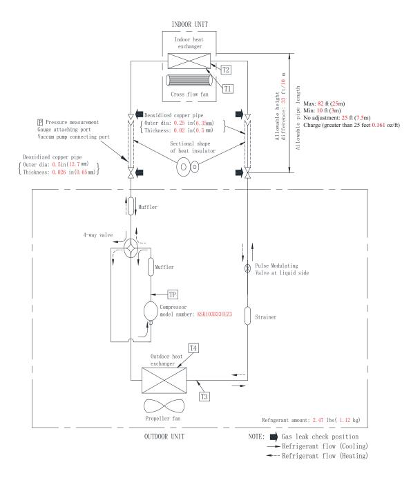
Fig. 14 — Refrigerant Cycle Diagrams 12K (115V)
