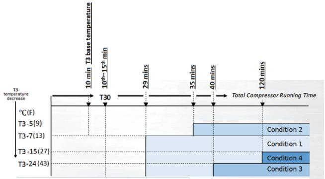
T3 - X (Y) means decrease in T3 base temperature by Celsius (Fahrenheit) degrees. e.g., T3-5(9) is a decrease of T3 by 5 degrees Celsius (9 degrees Fahrenheit).
