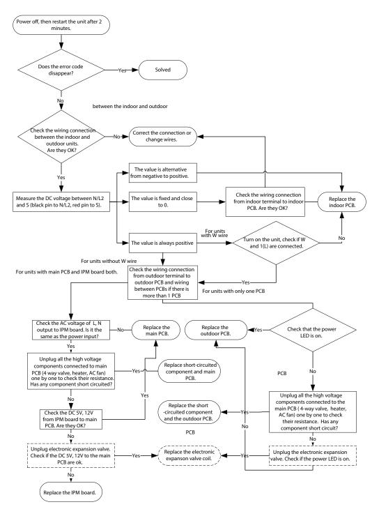
For certain models, outdoor PCB could not be removed separately. In this case, the outdoor electric control box should be replaced as a whole.
