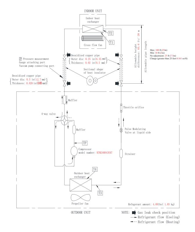
Fig. 17 — Refrigerant Cycle Diagram 18K (208/230V)
