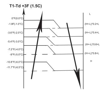
Fig. 32 — Auto Fan Action in HEATING Mode
