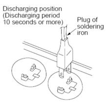
Fig. 37 — Discharge Position
