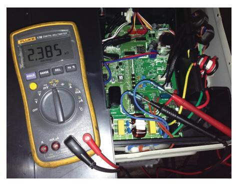
Fig. 47 — Use a digital tester to measure resistance
