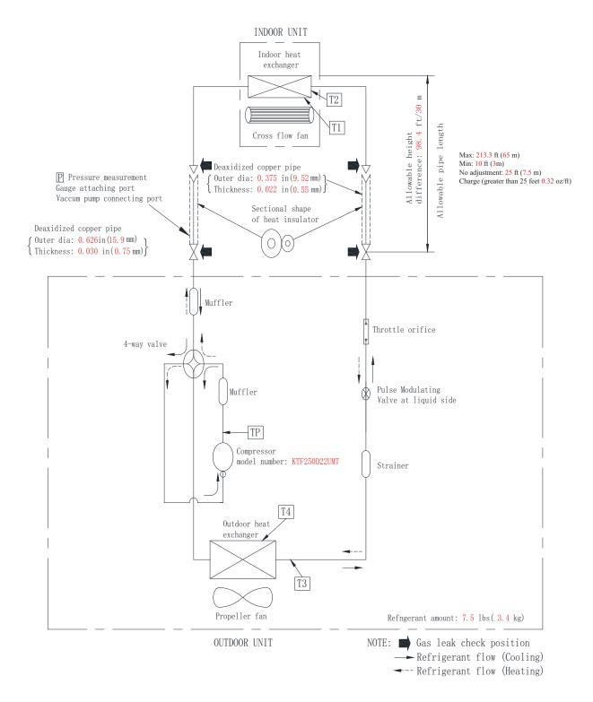
Fig. 20 — Refrigerant Cycle Diagram 36K (208/230V)
