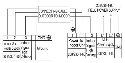
Fig. 8 — Connection Diagram 9K-12K (208/230-1-60 V)
