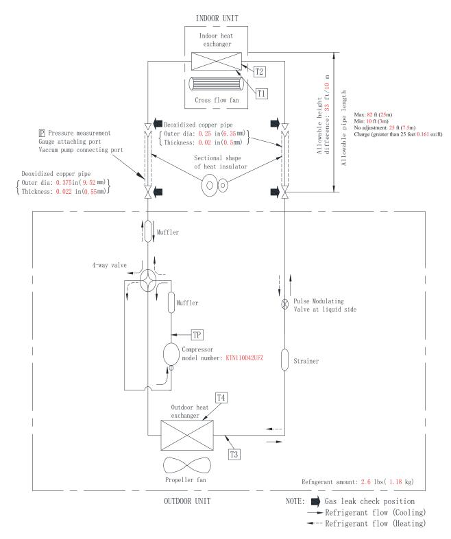
Fig. 15 — Refrigerant Cycle Diagrams 9K (208/230V)
