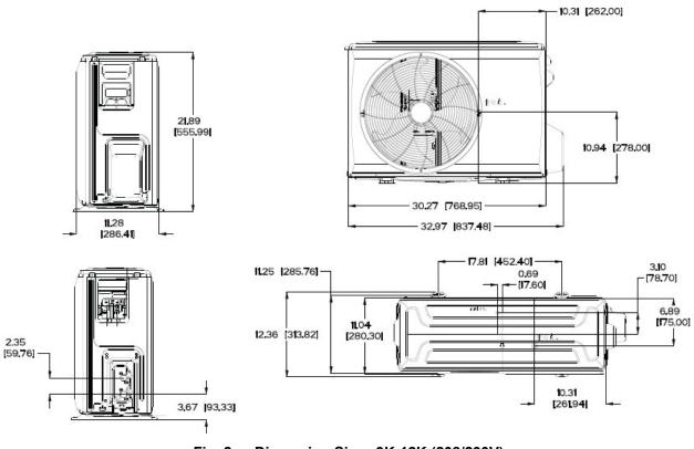
Fig. 2 — Dimension Sizes 9K-12K (208/230V)
