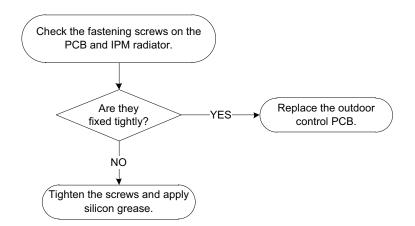
Top temperature protection for compressor or High temperature or High pressure protection of IPM module (PC02) (Cont)
