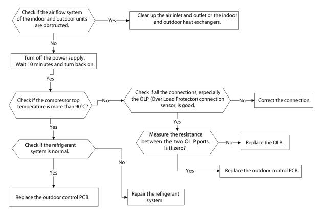
**NOTE:** For certain models, the outdoor PCB can not be removed separately. In this case, the outdoor electric control box should be replaced as a whole.
