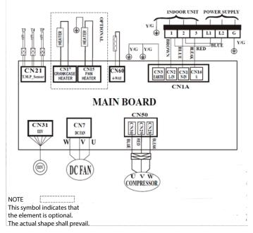
Fig. 11 — Wiring Diagram - Sizes 9-12K (208/230V)
