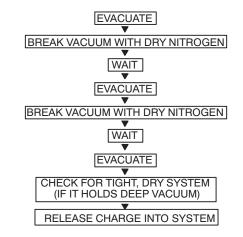
Fig. 24 — Triple Evacuation Method
