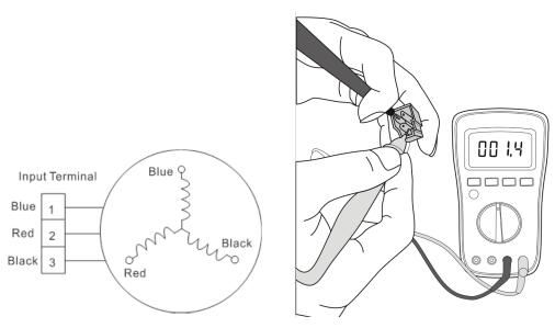
Fig. 42 — Compressor Checks
