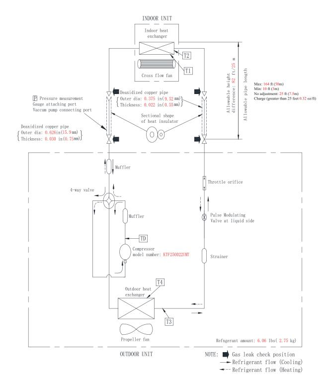
Fig. 19 — Refrigerant Cycle Diagram 30K (208/230V)
