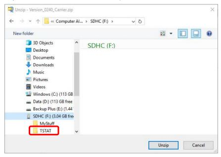
Verify that the files, including the BINF0431.hex file, have been extracted into the TSTAT folder of the MicroSD device. Note that the "USER" folder is where the photo and schedule files would be stored.
