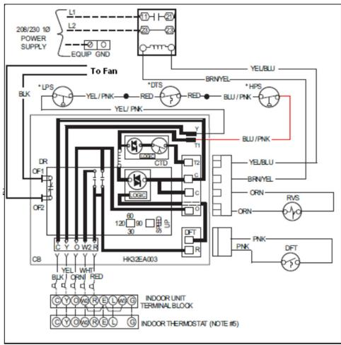
Original Board - Take BLU/PNK wire off of compressor contactor coil stake-on and move to T1 on the new board.
