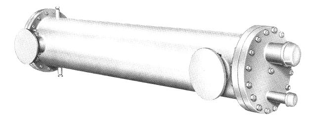
The 10RT shell-and-tube cooler assembly consists of a cooler, complete with refrigerant connections, water connections, thermowell connections, terne plated baffles, equalizer connections and 3/4-in. armaflex insulation. Basic assembly does not include expansion valves, solenoid valves, control thermostats or safety thermostats. Cooler is constructed and tested in accordance with the latest ASME code for unfired pressure vessels.
